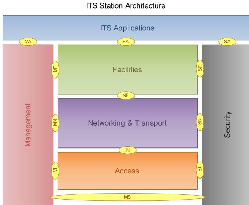
Figure 1: ITS station architecture (from ETSI EN 302 665 [1])
