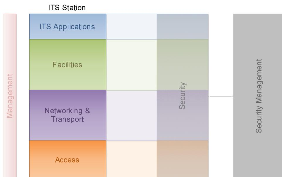
**Figure 3: Architectural ITS security layers**
