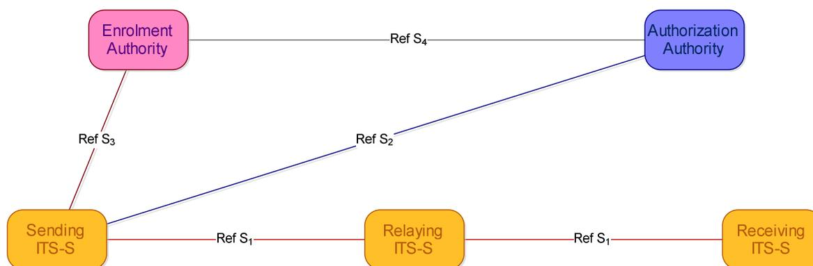
**Figure 9: ITS security reference model for DENM**
