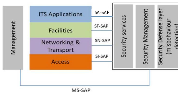
Figure 4: ITS-S security architecture: entities and interfaces
