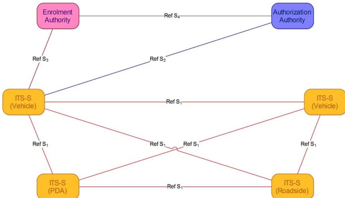
**Figure 7: ITS security functional elements and reference points**
