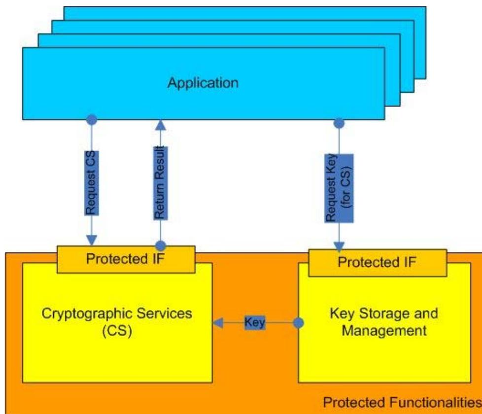
**Figure 10: Abstracted generic model of a Hardware Security Module (HSM) for ITS-S security**
