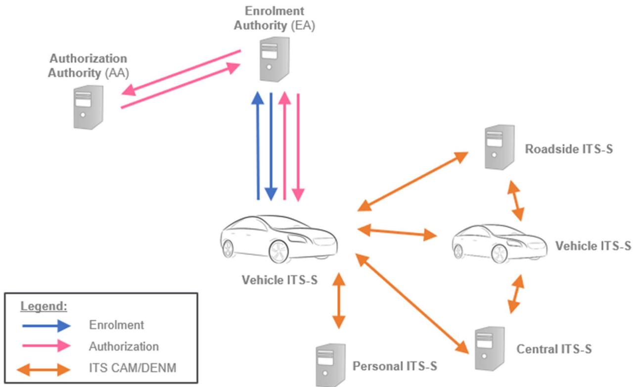
**Figure 6b: ITS communications reference scenario for butterfly AT provisioning**
