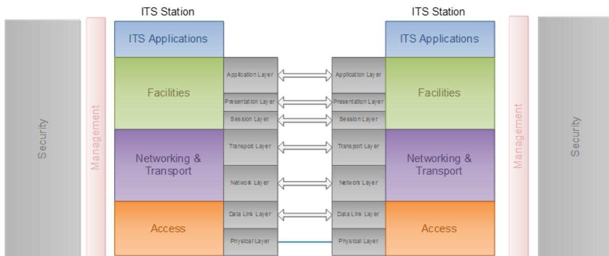
Figure 2: ITS communications architecture
