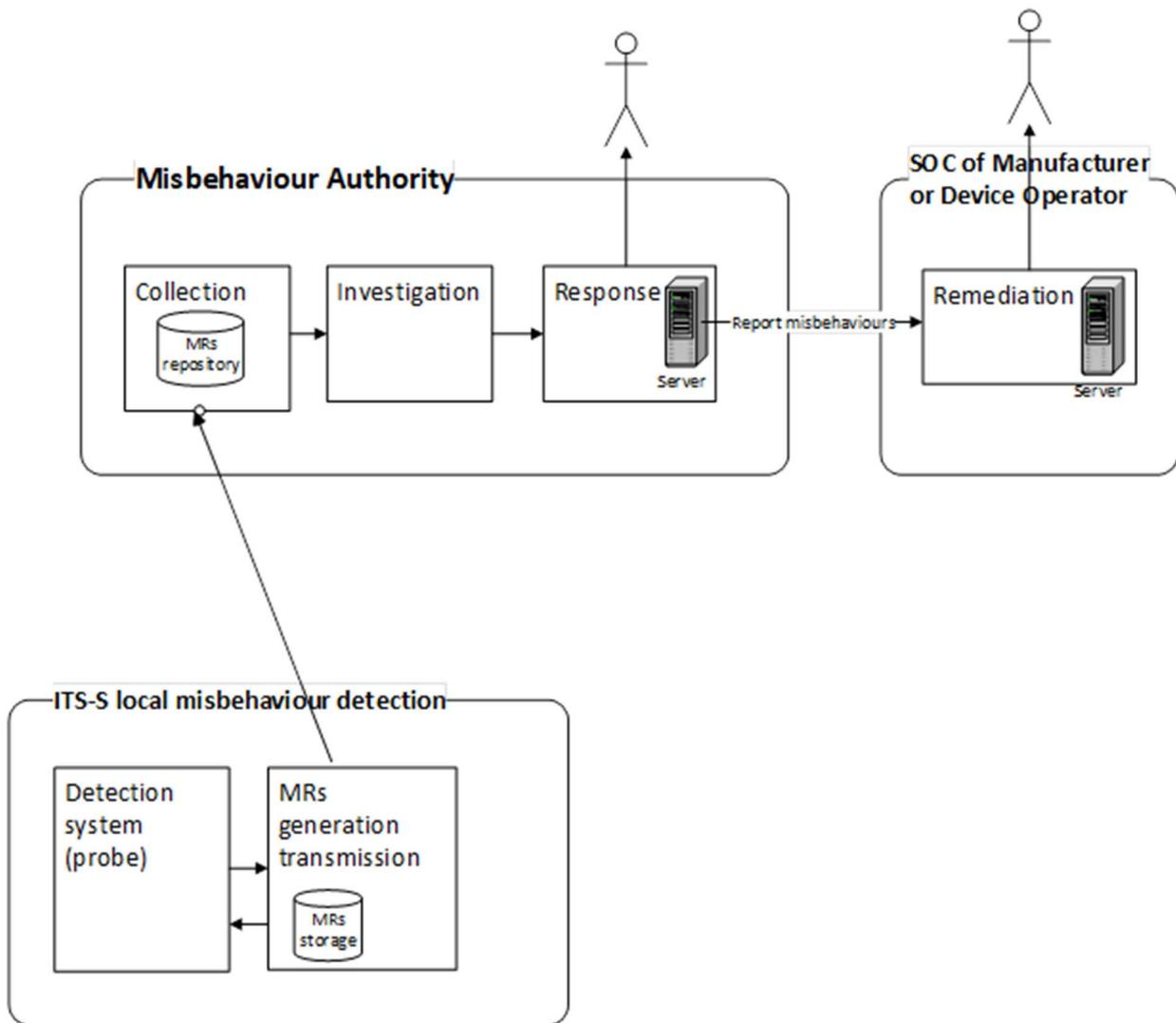
Figure 13: Misbehaviour detection management system
